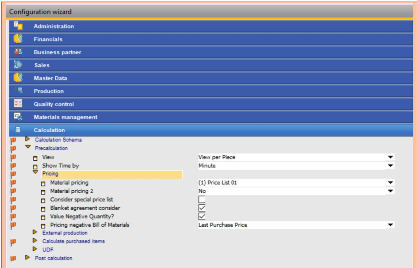
**Material Pricing:** Field used to specify the pricing of the materials when valuating assemblies.
